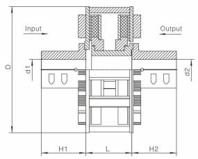
When the machine is overloaded or jammed, the air gap between the permanent magnet rotor and the conductor rotor increases rapidly until the maximum air gap, and the speed of the permanent magnet rotor at the machine end drops until it stops rotating, so as to realize the overload protection of the motor.
